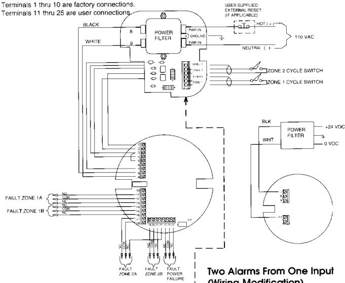
NOTE: Unit is shipped wired for use with 110 VAC power source. For use with 24 VOLT DC source, modify wiring as follows:
