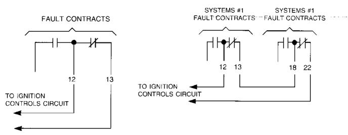
NOTE: Do not connect to high voltage. Connect to controls only.
