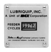
Counter housing clamps to a cycle indicator pin housing. A 6-digit mechanical counter, advanced by the movement of a divider valve cycle indicator pin, provides visual assurance that the system is functioning. Every "count" indicates one complete cycle of the divider valve assembly. Suitable for application at pressures up to 3500 PSI. Part number 527-002-410
