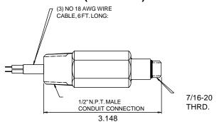
This ceramic-magnet switch is installed in place of a piston enclosure plug and detects the cycling divider valve piston as it moves back and forth.
