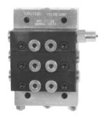
18 through 30 size MH divider valve sections are available with a factory-installed cycle indicator pin attached to either end of the piston. The pin moves in and out one time for each complete cycle of the divider valve assembly. Application pressure is limited to 3500 PSI.
