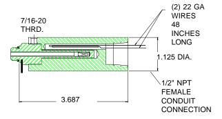
This magnetically operated SPST switch is installed in place of a piston enclosure plug. This "unattached pin" type switch can be used with any size MH working section
