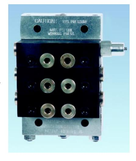
MH divider valves precisely proportion a volume of oil to satisfy the different requirements of every point in a lube system. They operate in sequential fashion to ensure that no point is missed. Series-Progressive design provides ready monitoring capability.
