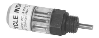
A No-Weep Magnetic Visual Cycle Indicator can be installed in place of a piston enclosure plug on any size divider valve section. Six steel balls in a transparent sleeve follow a magnet which moves with the cycling piston. Unlike a cycle indicator pin, working section displacement is not reduced. Suitable for application at pressures up to 7500 PSI. Part number 509-932-522.
