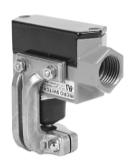
Switch bracket clamps to a cycle indicator pin housing. Cycle indicator pin movement repeatedly trips an electrical (limit) switch. Switch pulses provide input to a system controller which counts them to control and verify completion of the lube cycle.
